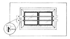
Metal window bars or grills fastened securely to the exterior of the foundation wall, or between the storm screen and window, or to the interior basement wall are the only truly effective means of giving basement windows proper security.
