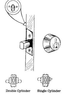
4. This lock is available with a double cylinder (key required to lock it from the inside as well as the outside). This is recommended for commercial applications only, not residential. Many fire prevention professionals warn that double-cylinder deadbolts create a health hazard in the event your family must flee the home quickly to avoid fire.
