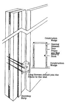
Although the opening between the wall and frame is braced at the top and the bottom with alignment wedges, the midsections are often left open, thus permitting the frame to bow under pressure. Solid blocks inserted between these openings will help to resist this form of attack.
